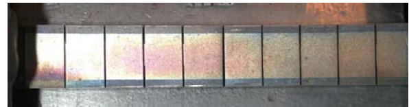
Figure 7: Mock-up after tests at 5 \text{ MWm}^{-2} , and a total of 2000 cycles.
