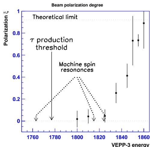
Figure 3: Measured Beam Polarization degree vs. VEPP-3 Beam Energy
