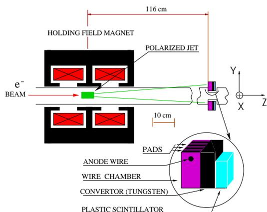
Figure 1: Lay-out of Møller Polarimeter with Internal Target.
