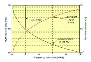
Figure 4: Expected MCP emptying time and equivalent input noise of the OPA657 avalanche photodiode preamplifier as a function of the system bandwidth.
