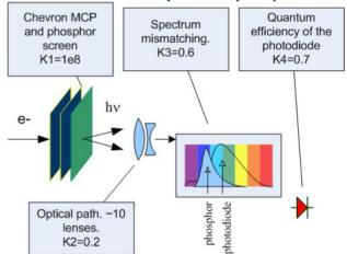
Figure 3: Transmission characteristics of the 'preelectronic' RGM stage.
