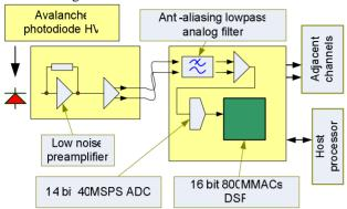
Figure 2: Single fast readout channel block diagram.
