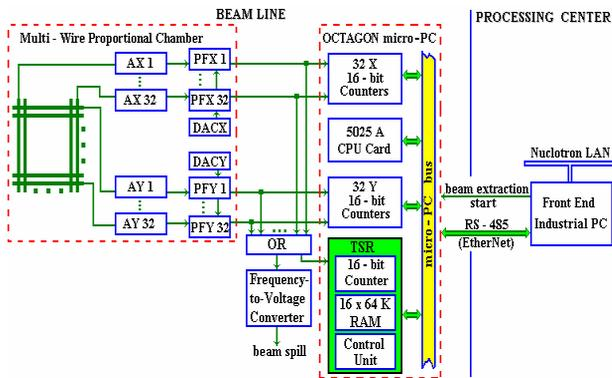
Figure 3: Block-diagram of the digital-mode MWPC electronics.
