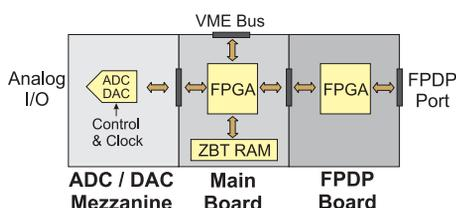
Figure 3: Layout of ADC and DAC board
