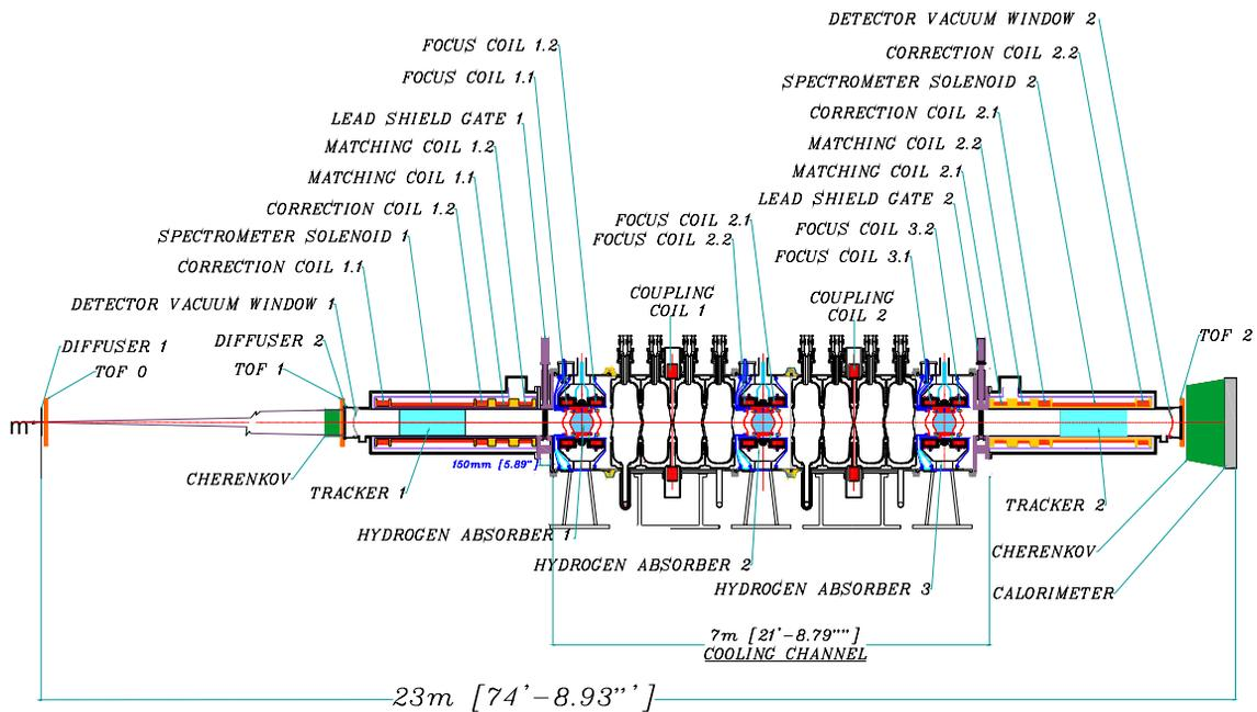
Figure 1: Layout of the MICE experiment.
