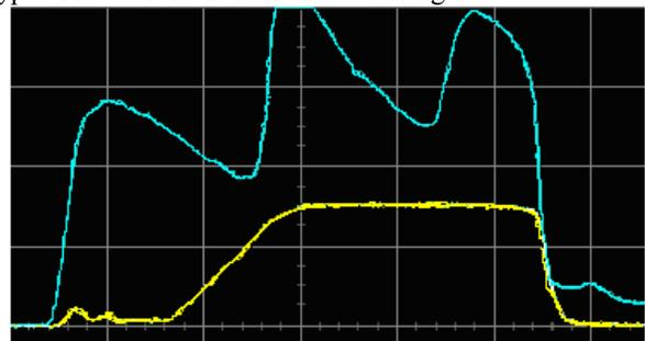
Figure 5: reflected RF power as a function of time (200 ns/div) in presence of a magnetic field; blue upper line, in PB1 and yellow lower line in PB2.
