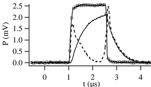
Figure 3: RF power in PB1 measured as a function of time; line with O points, incident klystron power; plain line, stored power in the cavity and dashed line stands for the reflected power at the input of PB1.
