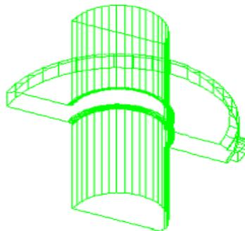
Figure 1: HFSS model of the copper pre-buncher.
