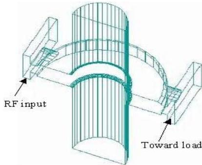
Figure 2: HFSS model of the second pre-buncher.
