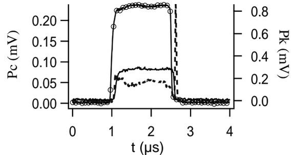
Figure 4: RF power in PB2 measured as a function of time; line with O points, incident klystron power (right axis); plain line, stored power in the cavity and dashed line stands for the reflected power at the input of PB1 (left axis).
