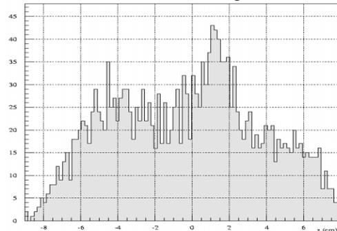
Figure 8: PARMELA simulation of the longitudinal profile (histogram) of the beam in the middle of PB1, beam energy is 140 keV and the current is 1.5 A.
