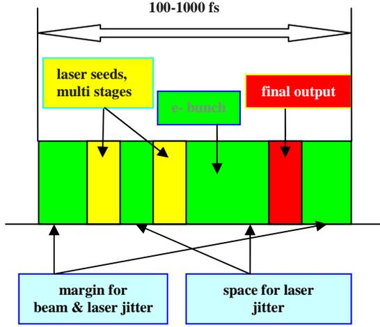
Figure 2: Arrival timing requirement of electron bunch and laser seed in the multi-stage HGHG process.
