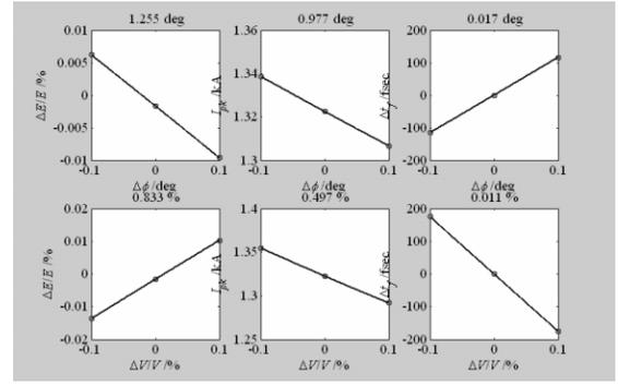
Figure 3: Sensitivities of beam quality to jitters in each section of linac (shown here is 2<sup>nd</sup> chirp linac section).
