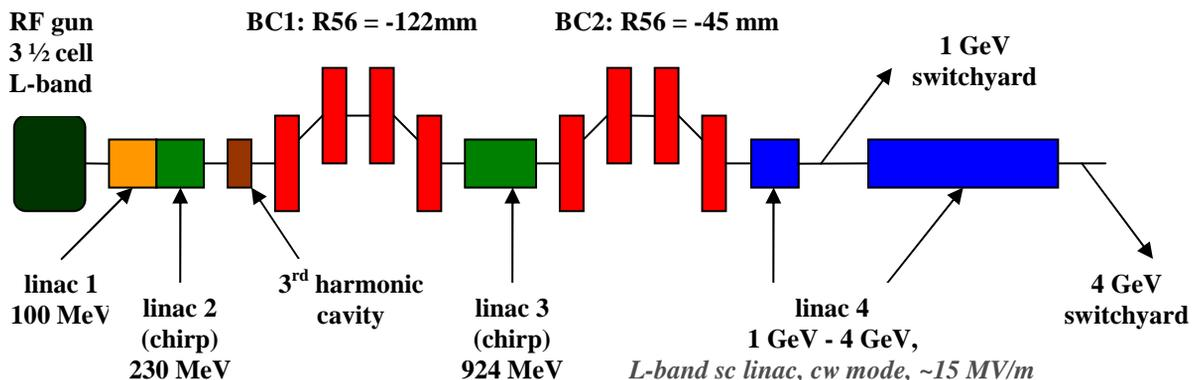
Figure 1: Layout of linac for the MIT x-ray FEL.
