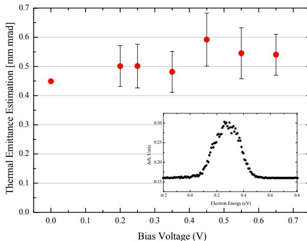
Fig. 2. Thermal emittance measured on Ag sample for a rms laser spot of 1 mm. The insert shows a typical spectrum of photoemitted electrons from Ag.
