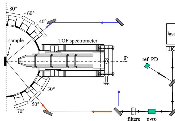
Fig.1. Sketch of the TOF analysis system. The sample is rotated at each angle to provide normal laser incidence.
