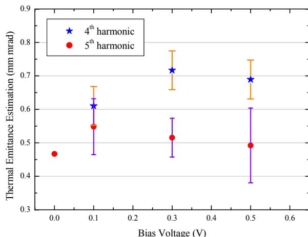
Fig. 3. Thermal emittance measured on a  $Cs_2Te$  sample at different bias voltages and at two wavelengths ( $\lambda = 264$  nm and 211 nm respectively for the 4<sup>th</sup> and 5<sup>th</sup> harmonic).
