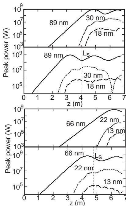
Fig. 3: Peak Power vs radiator length in the HGHH configuration.  $L_s$  represents the saturation length.
