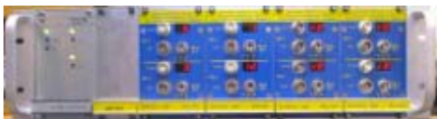
Figure 5: The 8 Channels Instrumentation Crate for PBPM Data Acquisition.
