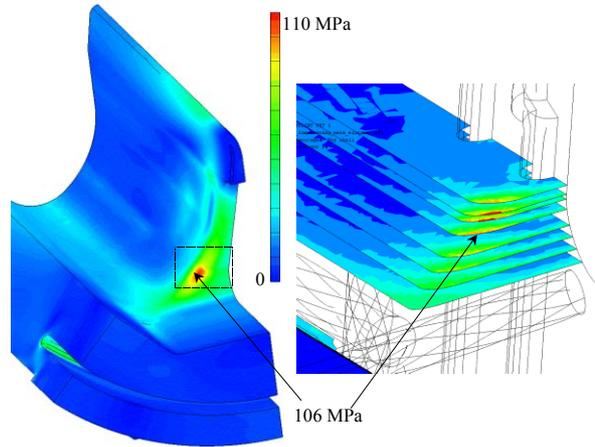
Figure 7. Stress on surface and in volume (cut planes).
