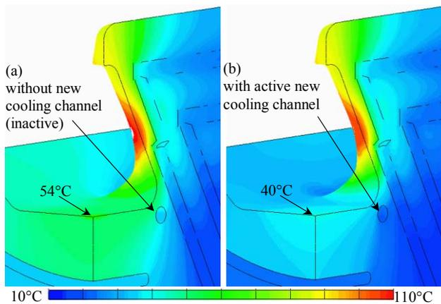
Figure 6. Effect of new cooling channel on temperatures.
