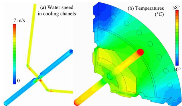
Figure 3. (a): Water speed in cooling channels; (b): temperatures in coupling plate and rod.
