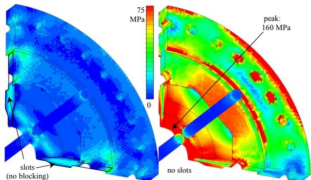
Figure 4. Stress in the coupling plate with/without slots.
