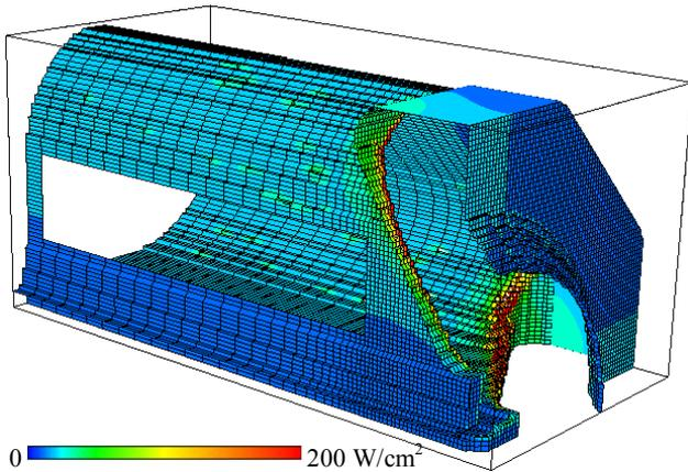
Figure 5. Power losses in RFQ output region.
