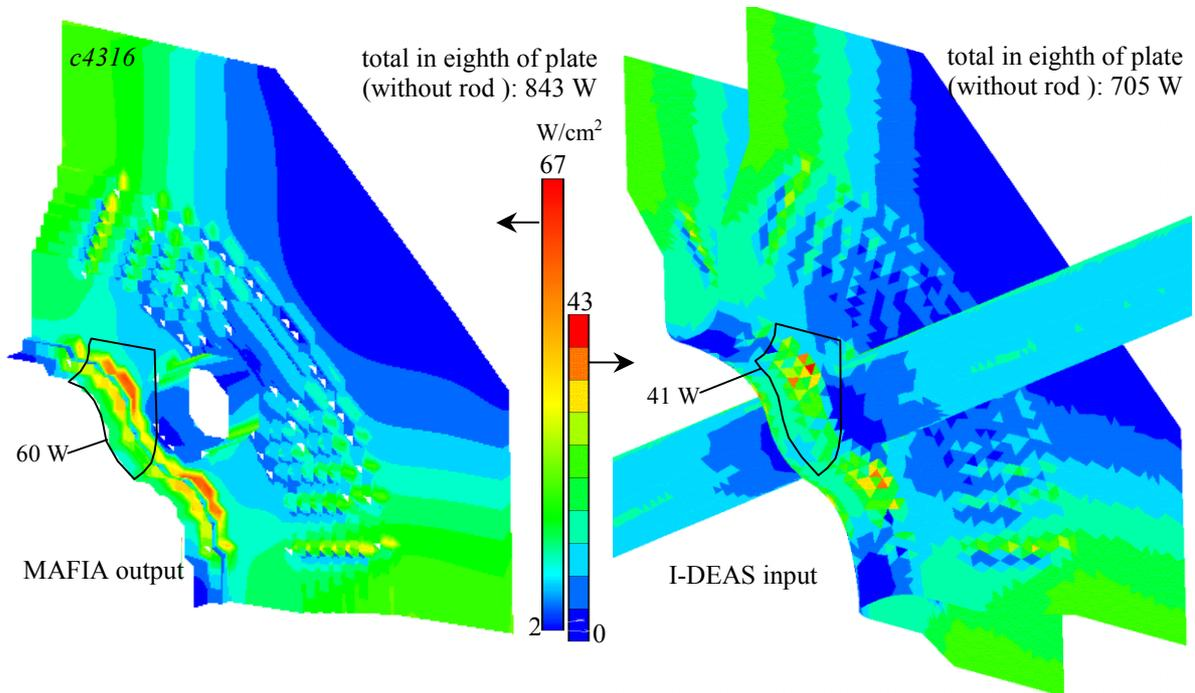
Figure 2. Power densities in the IPHI RFQ coupling plate transferred by MAPFLUX.
