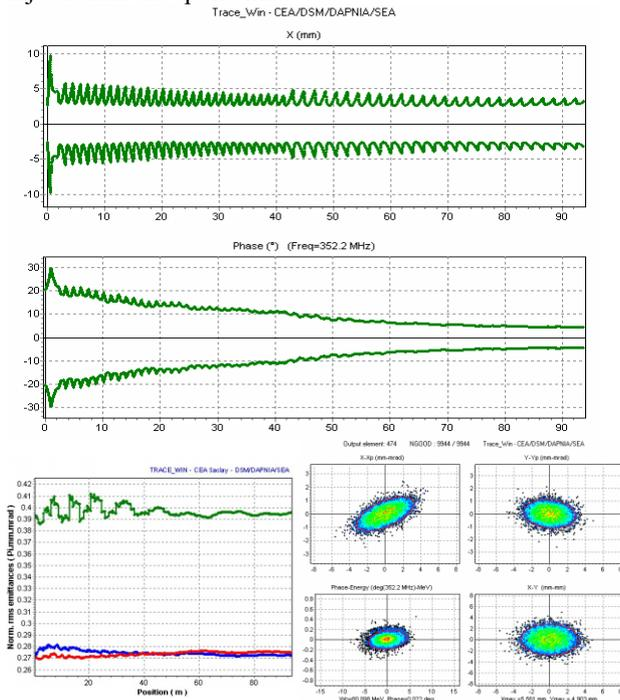
Figure 4: Simulation results for a matched beam: real beam envelopes, rms emittance evolution, and beam distribution at the linac exit (80 MeV).
