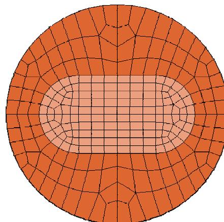
Figure 3: Cold mass FEM section.
