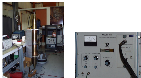
Figure 2. The beam position monitor test stand (left) used for measuring the accuracy and response of the various BPM's. The stand was driven by a variety of pulsers including a fast rise time pulser and a long pulse Velonex TM pulser with capabilities above one kilovolt and beyond six microseconds (left).
