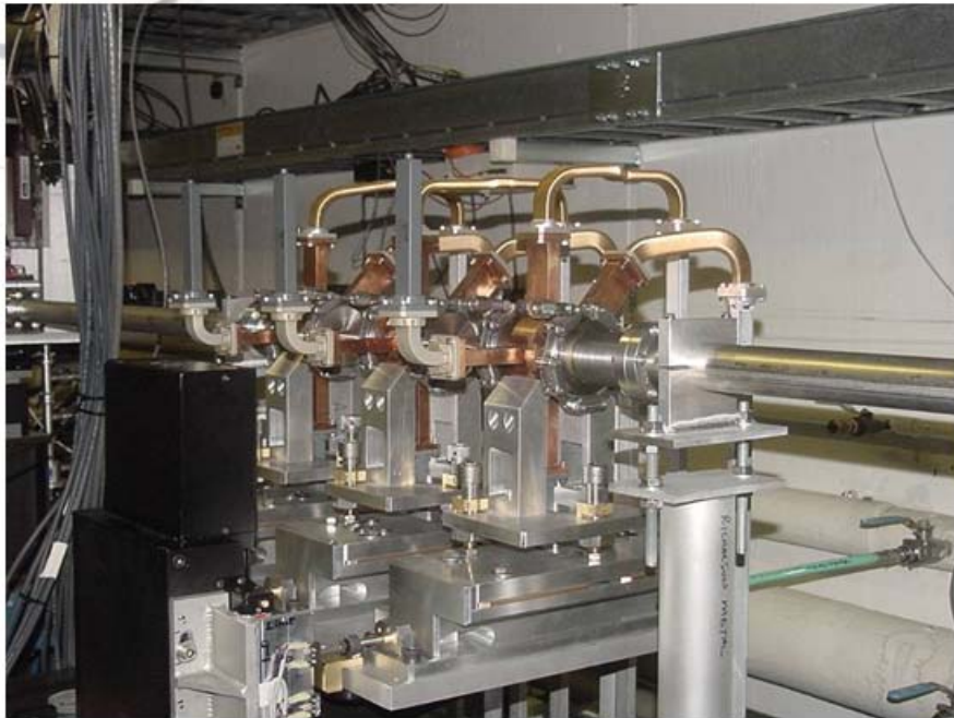
Test of 3 Cavity BPM at APS LEUTL
