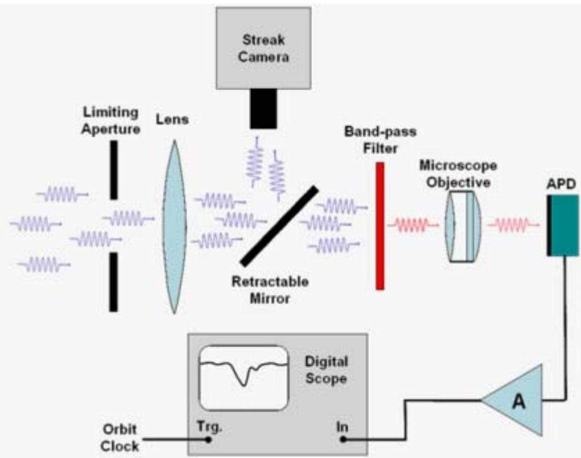
By using a bandpass filter with bandwidth  $\sigma_\omega$  and measuring the passage to passage relative variance  $\delta^2$  of the radiation intensity, the bunch length  $\sigma_\tau$  can be measured from:
