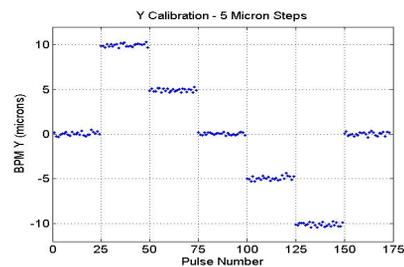
Figure 9: LCLS cavity bpm resolution measurement.
