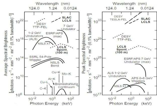
Figure 1: Average and peak brightness calculated for photon sources that are operating or under construction.
