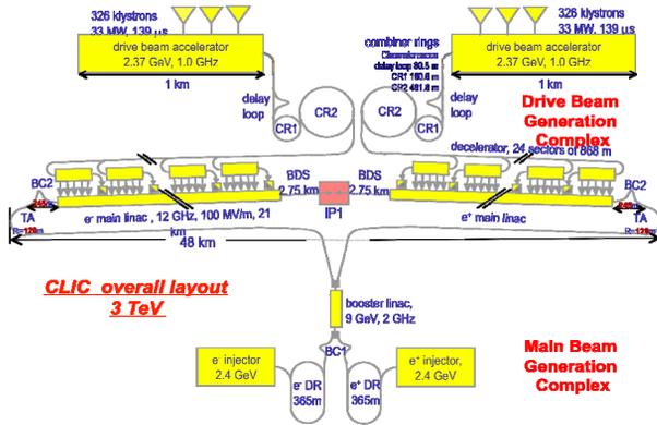
Figure 5: Schematic layout of CLIC.
