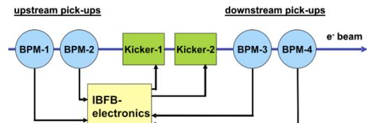
Figure 10: Proposed topology for XFEL intra-train feedback.
