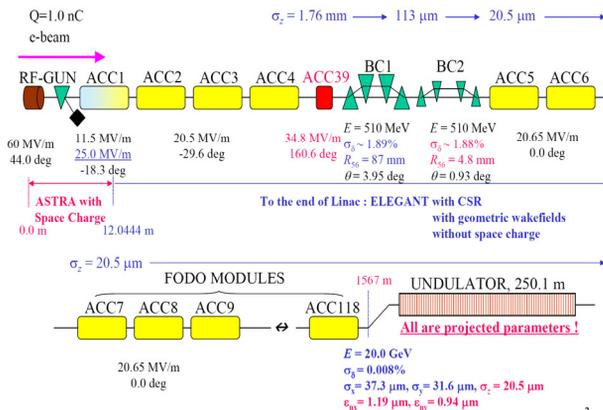
Figure 3: Schematic layout of the XFEL accelerator.
