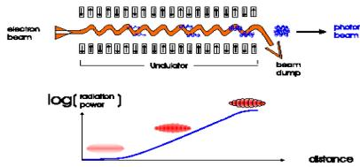
Figure 2: Principle of the FEL process.
