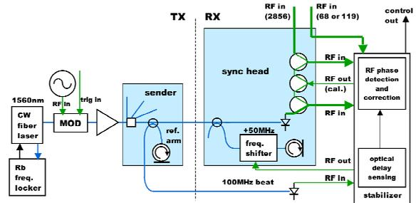
Figure 6: LBL optical RF distribution system.
