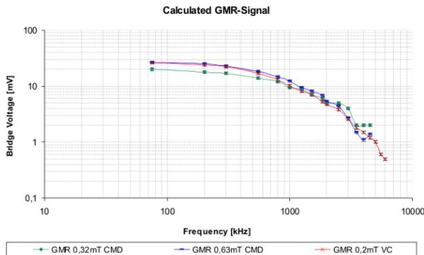
Figure 1: GMR signal vs. frequency.
