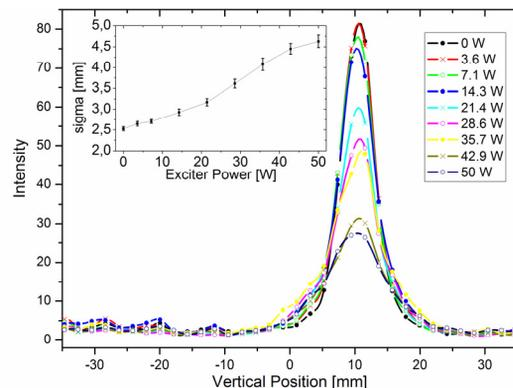
Figure 2: IPM measurements of vertical beam profile for different exciter settings. Insert: beam width sigma (Gaussian fit to beam profiles) vs. exciter power.
