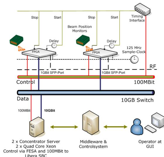
Figure 3: Layout of the new BPM data acquisition system for SIS18.
