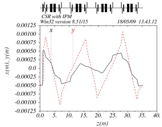
Figure 5: Closed orbit distortion of a 20 keV proton beam caused by the IPM voltage from MAD.
