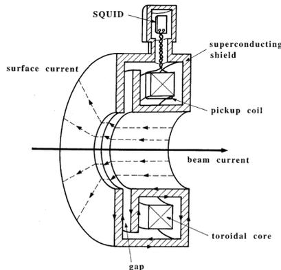
Figure 2: Principle of the CCC beam transformer [3].
