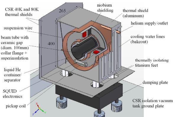
Figure 3: CCC beam transformer installation for the CSR.
