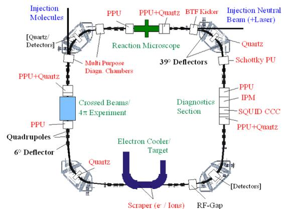
Figure 1: Layout of the CSR and diagnostics system.
