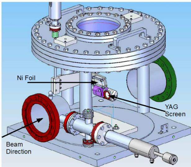
Figure 2: Temporary diagnostic assembly used in the measurements described in this paper.
