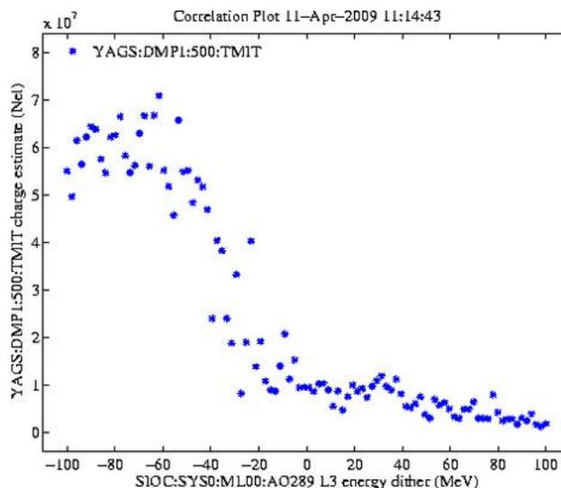
Figure 7: Energy scan of the FEL radiation, which is mostly 1st harmonic, incident on a 10- $\mu$ m nickel foil. This scan calibrates the machine energy in GeV and the strength of the undulator segment against the nickel  $K$ -edge, where the transmission drops.
