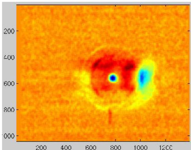
Figure 6: Difference image taken across the nickel  $K$ -edge. The dark central spot occurs coincides with the central rays from the undulator segment.
