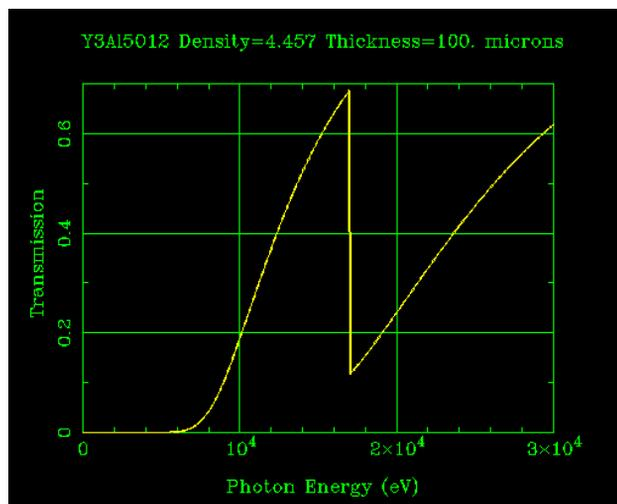
Figure 1: Transmission coefficient versus photon energy for YAG [2]. The yttrium  $K$ -edge occurs around 17 keV.
