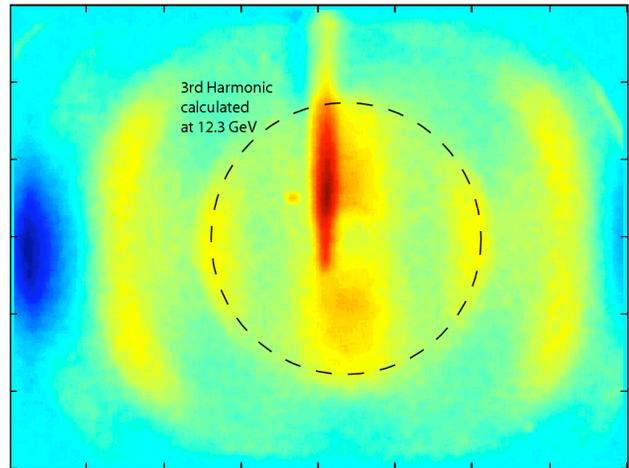
Figure 4: Difference of images taken with 12.3- and 11.3-GeV beams of spontaneous emission from one undulator segment. The dashed ring shows the predicted peak of 3rd-harmonic radiation, coinciding with the two partial rings in the image. Additional harmonics are also visible: the 2nd has two lobes above and below the middle, and the 5th harmonic appears as partial rings at higher angles.
