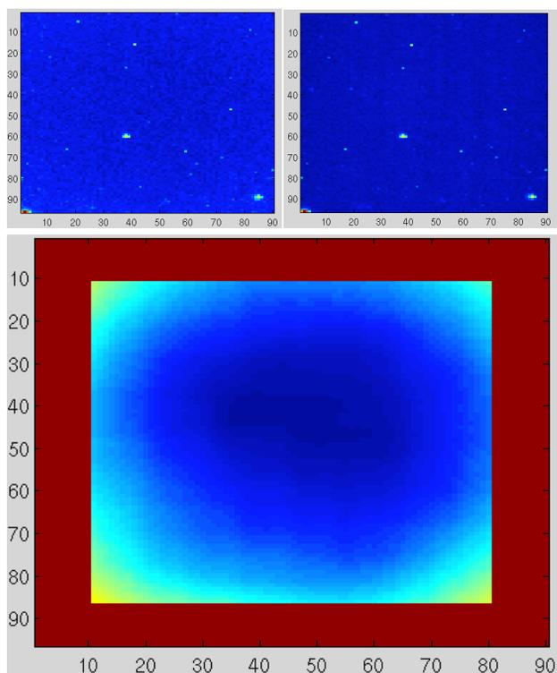
Figure 5: The upper two images were taken at slightly different electron energies corresponding to on-axis x-rays above (left) and below (right) the Ni  $K$ -edge. These are combined and filtered to produce a relatively clean image, shown enlarged in the lower frame, of only photons near the  $K$ -edge. The center of the resulting hole can be determined to within a few pixels.
