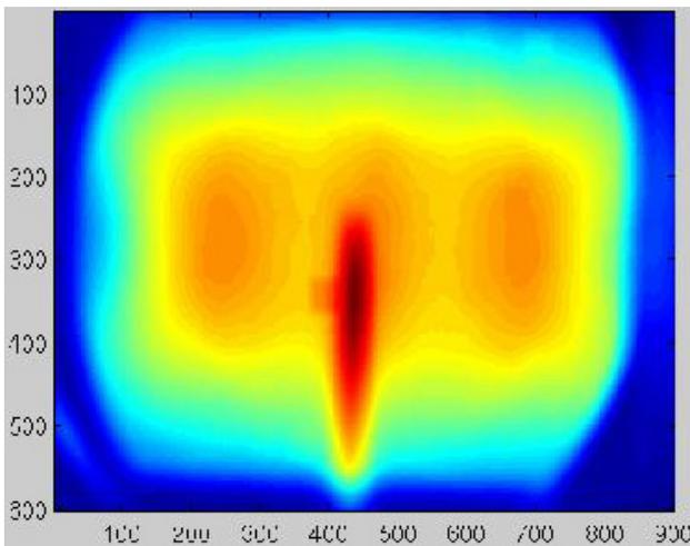
Figure 3: Spontaneous x-rays from one undulator segment as seen on the YAG crystal about 50 m downstream of the undulator. The central red stripe is caused by synchrotron radiation from the last dipoles. The three orange “humps” are the spatial signature of the 3rd harmonic.
