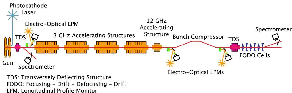
Figure 1: Schematic overview of the diagnostics for the 250 MeV Injector.
