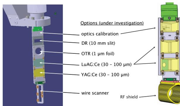
Figure 2: Screen holders for the low-energy diagnostic area (left) and the high-energy diagnostic areas (right). Several screens are available for the different operating modes.
