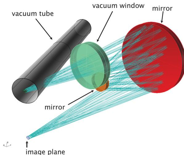
Figure 3: Offner reflective optics to image OTR over a wide wavelength range.
