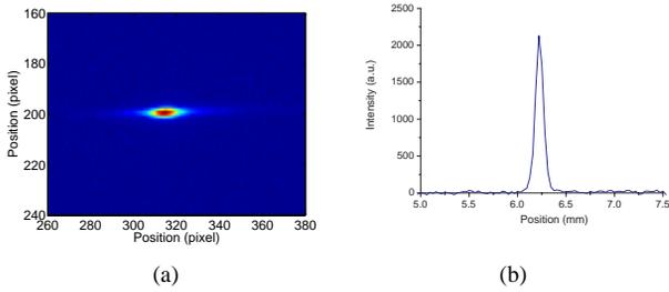
Figure 3: Vertical (a) beam waist of a typical beam and its projection (b) as the one analysed for the emittance measurement. The pixel calibration is  $31.25 \mu\text{m}/\text{pixel}$ .
