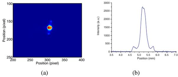
Figure 4: Beam with side structures in a region close to the vertical waist (a) and its projection (b). The pixel calibration is  $30.30 \mu\text{m}/\text{pixel}$ .
