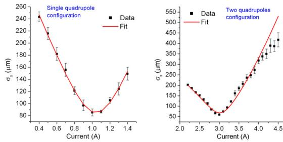
Figure 6: Quadrupole scan in single magnet and two magnets configuration. (200 pC, 7 ps FWHM pulse length and 145 MeV).
