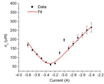
Figure 5: Quadrupole scan showing the effect of a beam with side structures (300 pC, 141 MeV).
