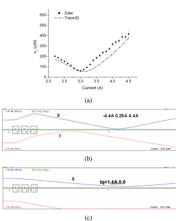
Figure 7: (a) Two magnets quadrupole scan compared to a TRACE3D simulation. (b), (c) Trace 3D envelope in the two quadrupole and single quadrupole configuration, respectively. The y axis extends from 0 to 0.6 mm for both x and y envelope curve. 200 pC, 7 ps FWHM pulse length and 145 MeV.
