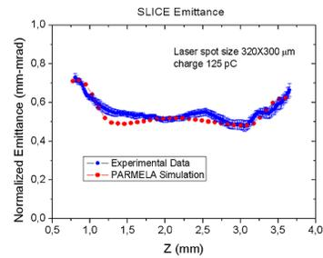
Figure 8: Slice emittance measurement compared to a PARMELA simulation. Z is the longitudinal position along the beam.
