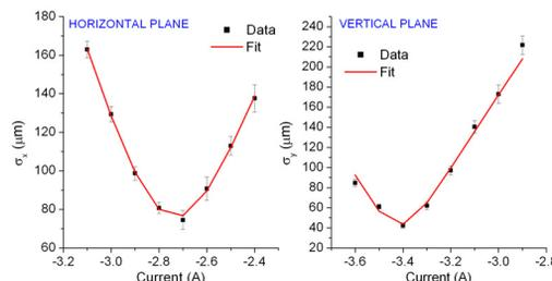
Figure 2: Comparison between the rms beam size measured at the flag  $F_1$  (black squares) and the one retrieved from the  $\chi^2$  minimization (red curve) as function of the quadrupole current (125 pC, 140 MeV).
