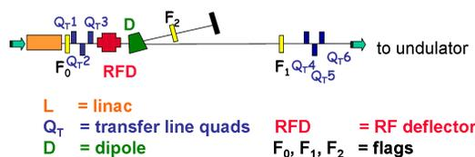
Figure 1: Layout of the high-energy experimental area.
