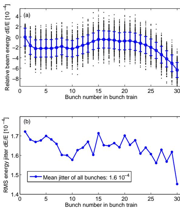
Figure 5: (a) Beam energy measured with the SR-PMT for 300 subsequent bunch trains with 30 bunches; (b) Corresponding rms energy jitter of each bunch.
