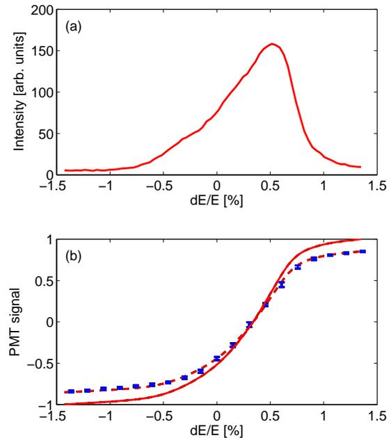
Figure 3: (a) Beam profile measured with the SR-camera; (b) Calibration curves of SR-PMT (dots) and deduced from beam profile (solid) with 8% crosstalk (dashed).
