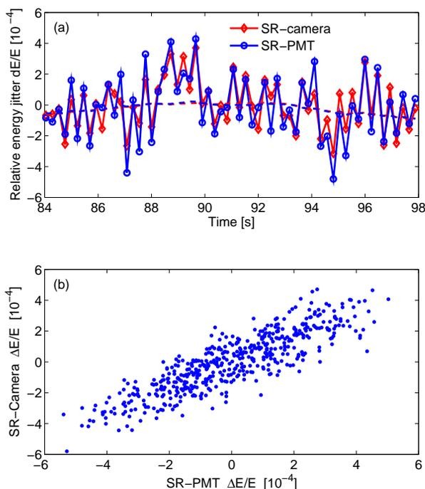
Figure 4: (a) Beam energy of single bunches measured with the SR-PMT and SR-camera for 60 subsequent bunch trains; (b) Correlation plot for 500 measurement points of the SR-PMT and SR-camera.
