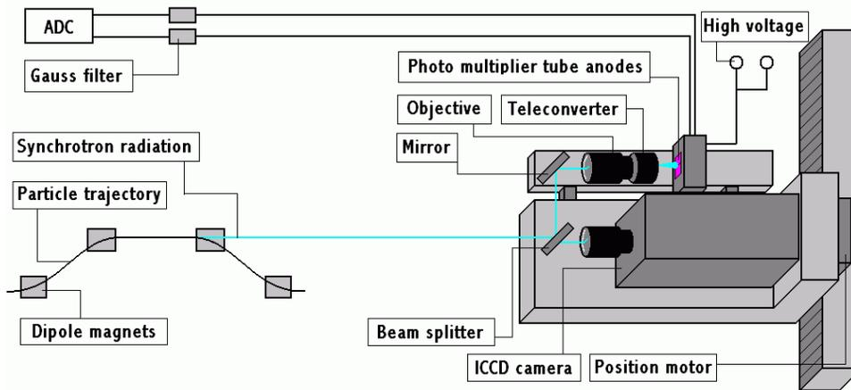
Figure 1: Schematic overview of the SR monitor setup. For further explanation see text.
