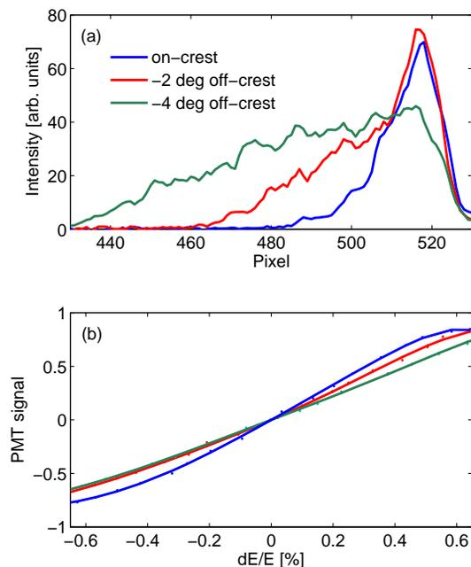
Figure 2: (a) Horizontal beam profiles measured with the SR-camera for 3 ACC1 phases; (b) Corresponding energy calibration of SR-PMT signal.
