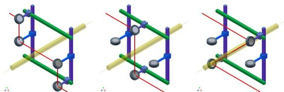
Figure 3: Three possible mirror configurations. The mirrors can rotate about their centrelines and move along  $x$  or  $y$ , depending on their positioning. The laser beam is shown in red and the ion beam in yellow
