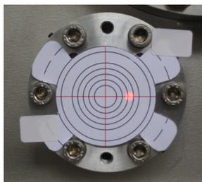
(b) A target mounted on the output window. The target's radii are 5 mm, 7.5 mm, 10 mm and so on. The movable stages are nearest to the vessel wall that the windows are mounted in (i.e. this is the configuration with the extra path length is 400 mm). Note that the spot has moved by  $\sim 7$  mm, compared to its position in Figure 5b.
