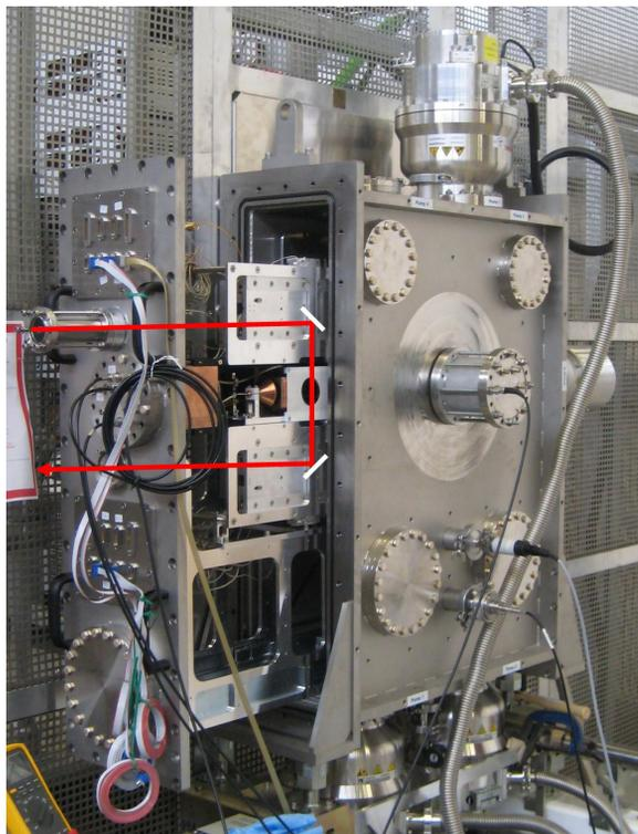
Figure 4: The vacuum vessel and the components required to make the beam density distribution measurement. In the centre of the picture the detector's copper Faraday cup can be seen. The central position of the mirrors is shown schematically in white, with the corresponding laser path in red.
