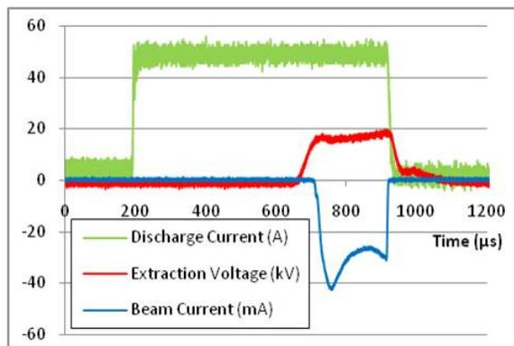
Figure 1: An oscilloscope trace of the first beam from the FETS ion source [1]
