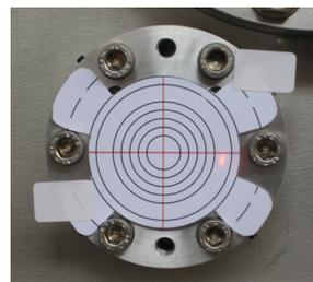
(c) For this picture the stages were moved to the furthest position from the vessel wall with the windows mounted in (such that the extra path length is 400 mm). Note that the spot has moved by  $\sim 7$  mm, compared to its position in Figure 5b.
