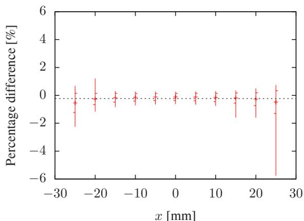
Figure 7: The discrepancy between the simulated and measured values of the  $x$ -component of the dipole's field. Each measurement was compared to the simulated value at its position and then the discrepancies in each  $x$ -plane were averaged. The crosses show the average percentage difference for each plane; the ticks,  $\pm 1\sigma$  from the average point; and the extent of the lines, the maximum discrepancies.
