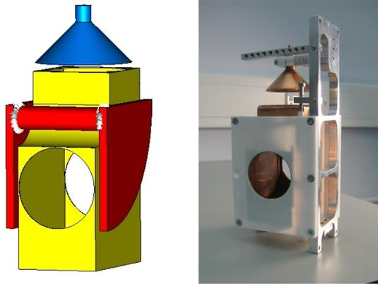
(a) A schematic of the detector. The magnet is shown in red, the accelerating sheath in yellow and the Faraday cup in blue.
