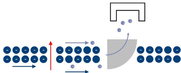
Figure 2: An illustration of the laser-based profile monitor principle. The laser (red) detaches some electrons (light blue) from the  $H^-$  ions (dark blue), which are then deflected by a dipole magnet (grey) into a Faraday cup.
