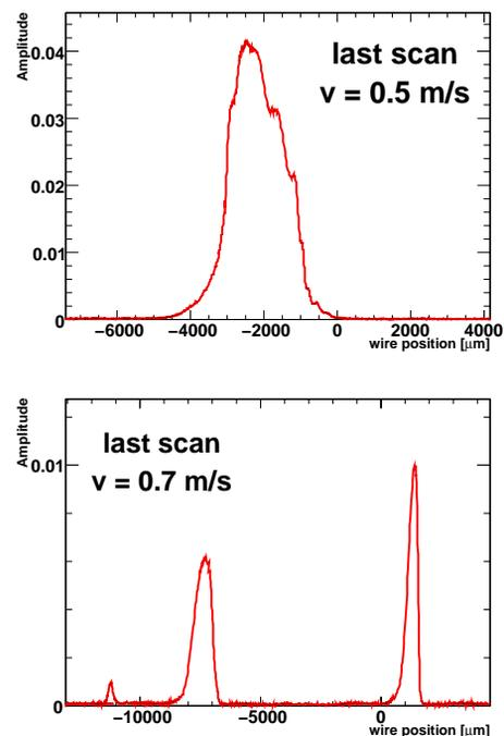
Figure 1: The last profiles after which the wire has been found broken. Upper plot shows breakage of vertical wire: deviations from Gaussian profile are visible. The bottom plot shows breakage of the horizontal wire: multiple peaks suggest that the wire has already fragmented.
