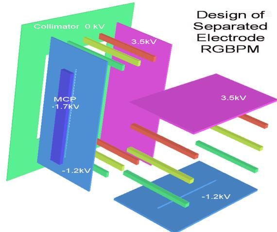
Figure 5: Calculated construction of the RGBPM-2 with the relevant voltages shown on the electrodes.
