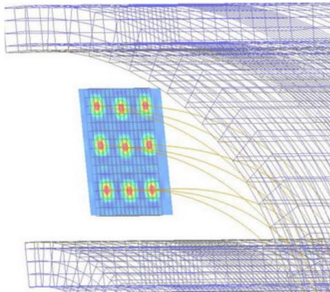
Figure 3: Projection of different beam positions onto the MCP of the RGBPM-1.
