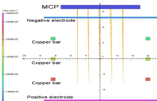
Figure 7: Twenty five particles, starting on a 30 mm x 30 mm XY-grid are tracked through the calculated electric field of the vertical profile monitor of RGBPM-2. The distortion of the profile is about 1mm due to non homogeneity of the electric field.
