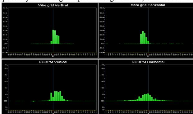
Figure 4: The horizontal and vertical RGBPM-1 profiles, bottom, compared with the profiles measured with a wire grid on top.
