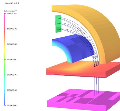
Figure 2: Calculated ion paths in the electrostatic fields of RGBPM-1.
