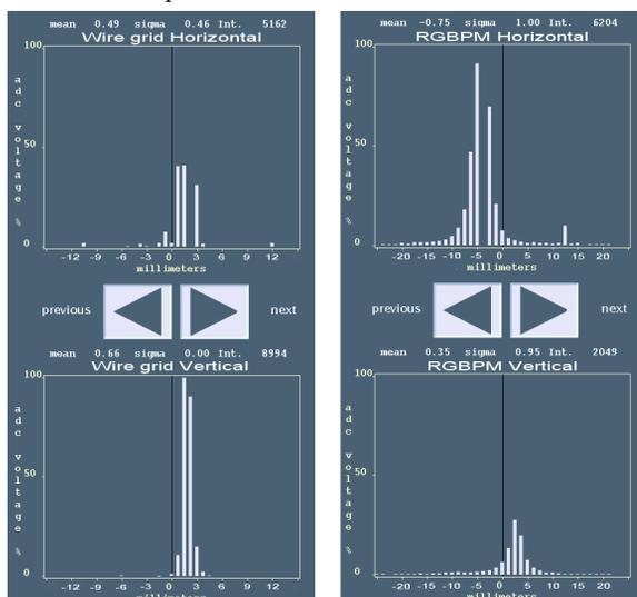
Figure 8: The profile of a 60 nA beam of 99 MeV oxygen ions measured with the grid is shown on the left. The profile measured with the RGBPM-2 is shown on the right.
