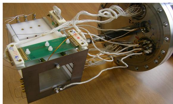
Figure 6: The residual gas beam profile monitor RGBPM-2. The 50 x 50 mm<sup>2</sup> opening for the beam is defined by a square tantalum protection screen in front of the monitor.
