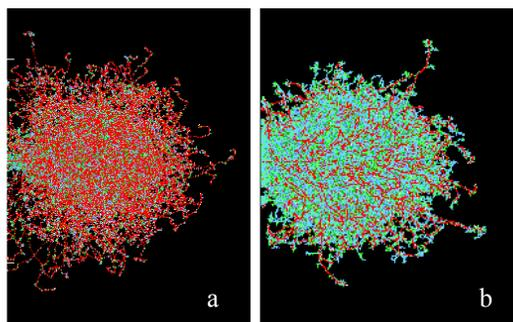
Figure 3: TRIM simulation of Helium (a) and Carbon (b) ion impinging into SiO<sub>2</sub> at 8 keV/u with the total number of ions equal to 1000. The longitudinal range and straggle (in parentheses) of Helium and Carbon are 866 Å (133 Å) and 282 Å (133 Å).
