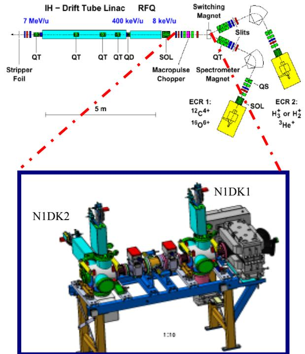
Figure 1: The Low Energy Beam Transport at HIT and the position of the Pepper-Pot Scintillator Screen device within the LEBT.
