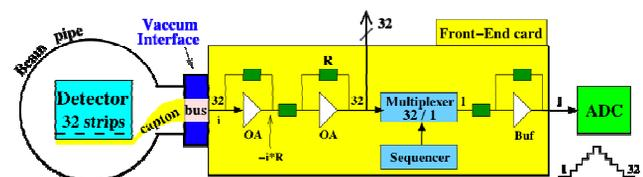
Figure 2: Front-end electronic sketch.
