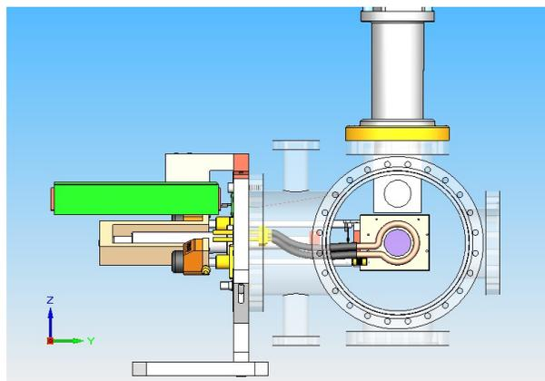
Figure 5: In horizontal, the monitor mounted on a piston, with its front-end electronic card on the left (green). In vertical, the SEM grid profiler is shown.
