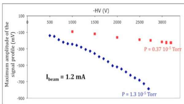
Figure 4: Maximum amplitude response for a 1.2 mA beam intensity at 2 vacuum pressures.
