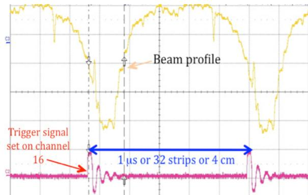
Figure 3: Beam profile seen on an oscilloscope every 1060 ns, which correspond to the 32 strips, lay out over 40 mm.
