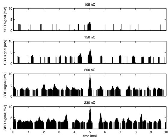
Figure 4: SBD signal (60-90 GHz, unamplified) for increasing single bunch charge with low-alpha optics.
