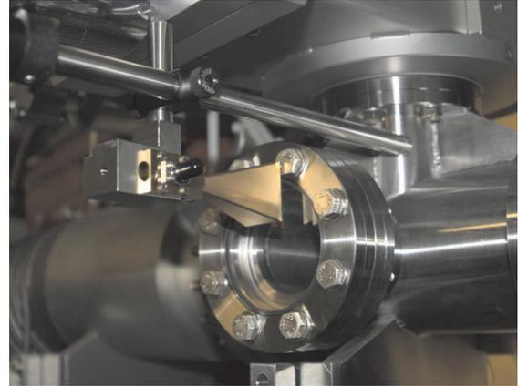
Figure 1: Photo of the 60-90 GHz detector with horn antenna mounted next to the visible light extraction.
