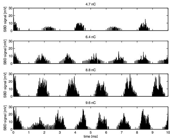
Figure 3: SBD signal (60-90 GHz, unamplified) for increasing single bunch charge with normal optics.
