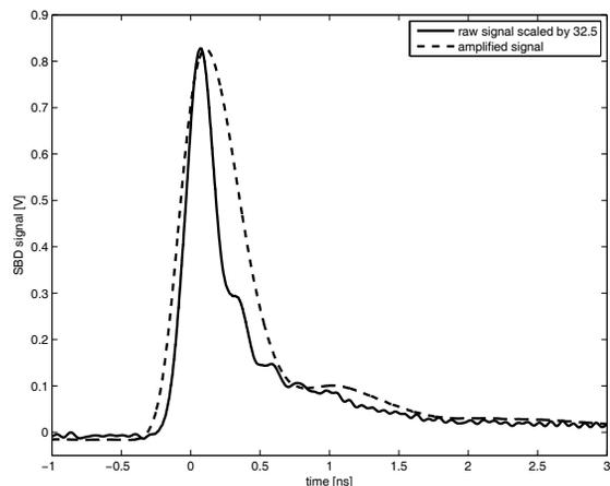
Figure 2: Pulse shape from 30-50 GHz detector without and with amplifier. Both traces are averages of 512 acquisitions triggered only on strong pulses.
