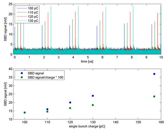
Figure 7: SBD signal (30-50 GHz, amplified) from every turn of an increasing single bunch in low-alpha optics.
