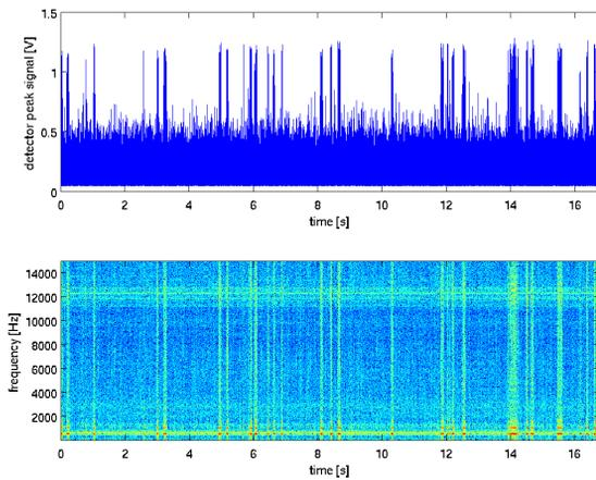
Figure 5: SBD signal (30-50 GHz, amplified) shows rare strong bursts with continuous weaker bursts between. Colour coded spectrogram is generated from block FFT of 2048 points at 500 kS/s.
