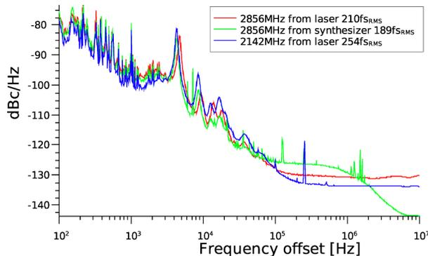
Figure 2: Phase noise spectra of the RF reference signals with integrated absolute jitter (from 100 Hz to 10 MHz).
