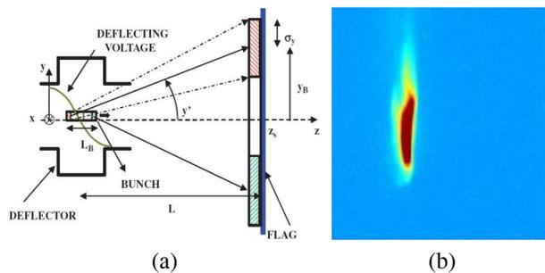
Figure 6: (a) Sketch of the RF deflector working principle and (b) an acquired image showing the longitudinal beam shape.
