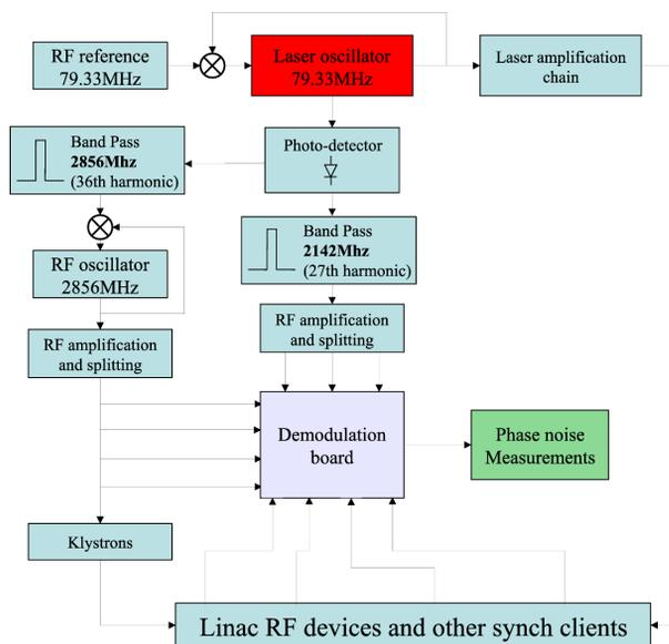
Figure 1: Layout of the synchronization system of SPARC.
