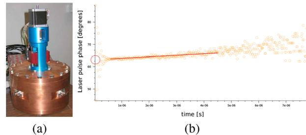
Figure 4: (a) Picture of the resonant cavity for the LAM and (b) an acquired phase data for a single UV pulse with emphasis on the analysis algorithm.
