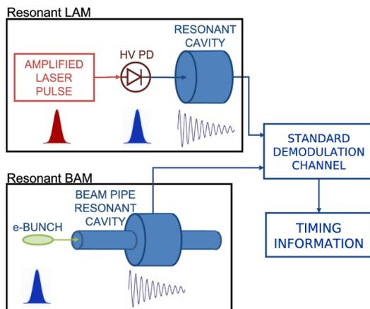
Figure 3: Block diagram of the BAM and LAM devices.
