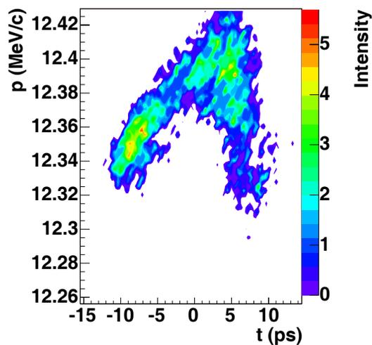
Figure 3: Measured longitudinal phase space distribution for a gradient of 60 MV/m at the cathode, gun phase of maximum momentum gain and booster phase of maximum momentum gain  $-10^\circ$ .
