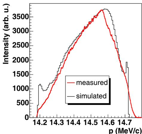
Figure 2: Comparison of measured and simulated momentum distribution for a charge of 250 pC, a gradient of 60 MV/m at the cathode, gun phase of maximum momentum gain  $+10^\circ$  and booster phase of maximum momentum gain  $+10^\circ$ .
