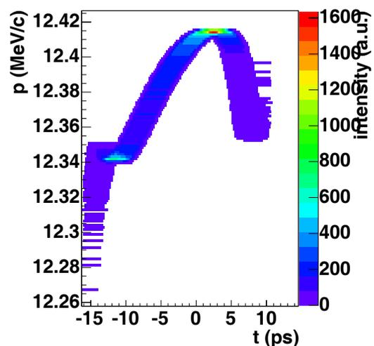
Figure 5: Simulated longitudinal phase space distribution for a gradient of 60 MV/m at the cathode, gun phase of maximum momentum gain and booster phase of maximum momentum gain  $-10^\circ$  convoluted with the resolution of the streak camera.
