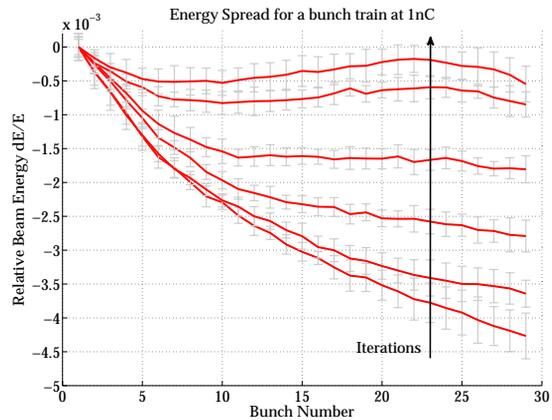
Figure 3: Removing beam induced RF field deviations along the bunch train with a learning FF algorithm.
