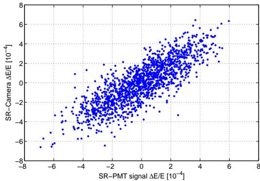
Figure 2: Correlation plot for 500 bunches recorded simultaneously with the SR-PMT and SR-camera.
