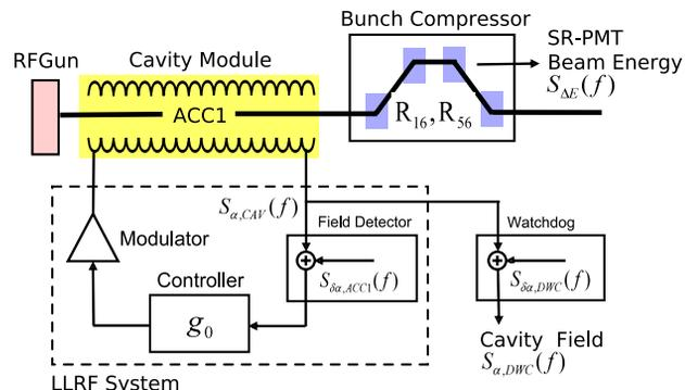
Figure 1: Schematic of FLASH injector.
