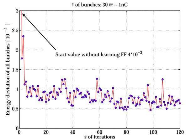
Figure 4: Minimization of the rms energy deviation of all bunches within a bunch train by applying the learning FF algorithm.
