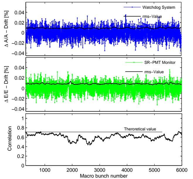
Figure 5: (top) Cavity vector-sum field amplitude fluctuations measured with the watchdog system, (middle) beam energy fluctuations measured with the SR-PMT, (bottom) correlation between watchdog system and SR-PMT.
