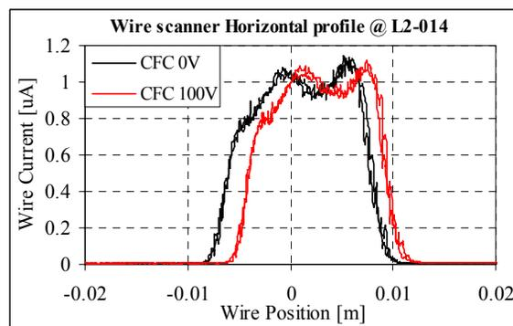
Figure 7: CFC polarisation effect on H<sub>3</sub><sup>+</sup> beam profiles.
