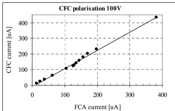
Figure 6: CFC current at different H<sub>3</sub><sup>+</sup> beam intensity.
