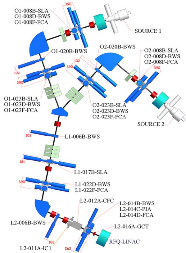
Figure 1: LEBT Instrumentation Layout with elements names. SLA are Slits, BWS are Wire Scanner in both planes, FCA is Faraday Cup, CFC is the Chopper Faraday Cup, PIA is Profile Grid, GCT is a current transformer and IC1 is the electrostatic chopper.
