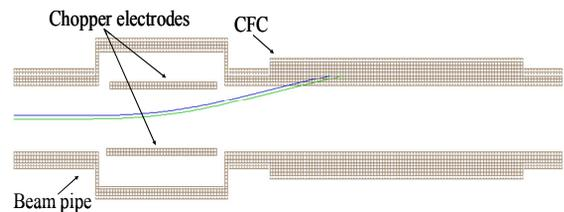
Figure 4: CFC Simion Code 7.0 simulation, top view: chopper electrodes polarized at ΔV=4kV.
