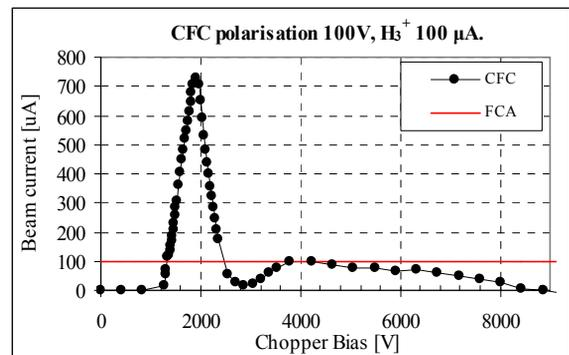
Figure 5: CFC measured current at different chopper deflection voltages (Chopper Bias [V] on abscissa) with a H<sub>3</sub><sup>+</sup> probe beam of 100 µA.
