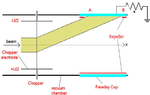
Figure 2: Schematic top view of the CFC working principle.
