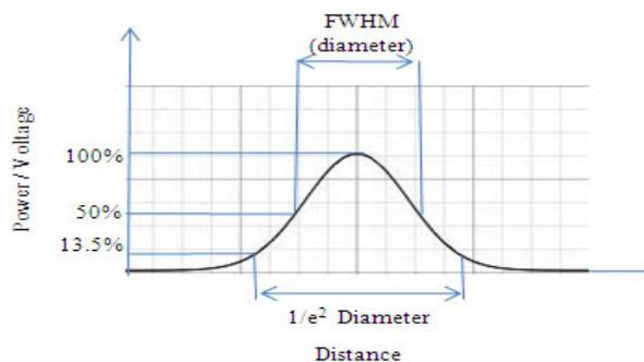
Figure 5: Typical Gaussian curve.
