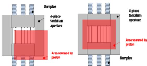
Figure 3: Beam alignment procedure.
