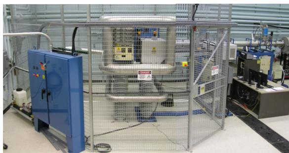
Figure 2: NEC's 400 kV ion implanter.
