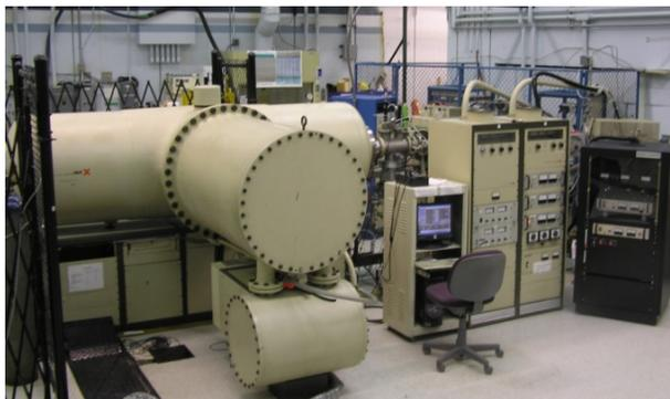
Figure 1: 1.7 MV Tandetron accelerator.
