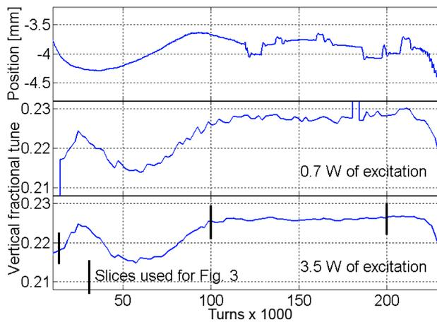
Figure 2: Vertical beam position and fractional tune, see text for beam parameters. Excitation at  $q_{ex} = 0.23 \pm 0.05$  with amplitudes of  $P_{ex} = 0.7$  W for middle graph and  $P_{ex} = 3.5$  W for lower graph.
