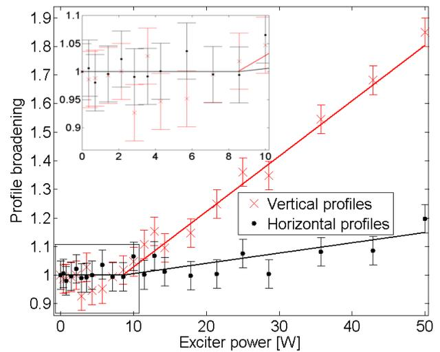
Figure 6: The increase of the standard deviation of beam profiles is shown as a function of exciter power. Points represent a mean value of 200 beam profiles of IPM, recorded at the end of the ramp.
