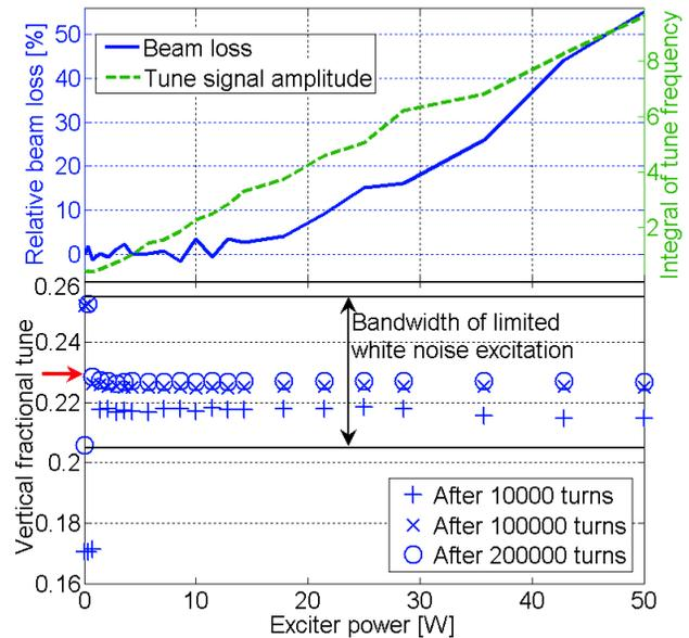
Figure 3: Beam response on noise excitation for dedicated times on ramp. Red arrow in lower part marks the machine preset tune value.
