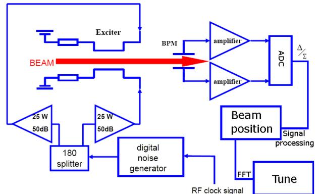
Figure 1: System schematics. The Beam Position Monitor is read out using a fast ADC. A white noise generator with limited bandwidth is connected to an exciter.
