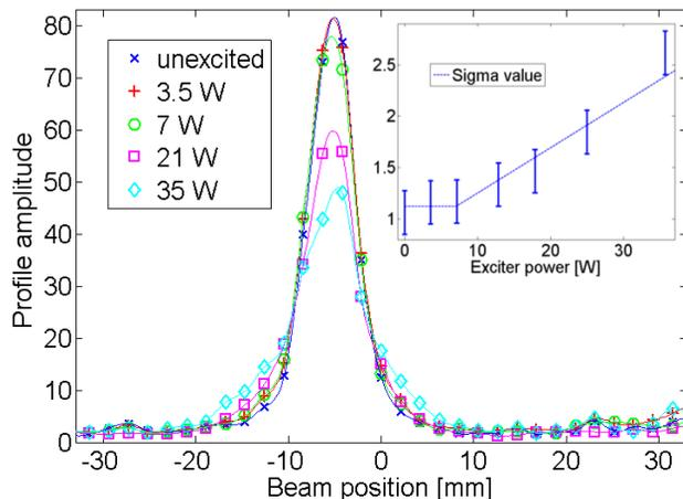
Figure 5: Vertical beam profiles of  $\text{Ar}^{18+}$ -beam measured by an IPM. Profile alteration by increasing exciter power is shown.
