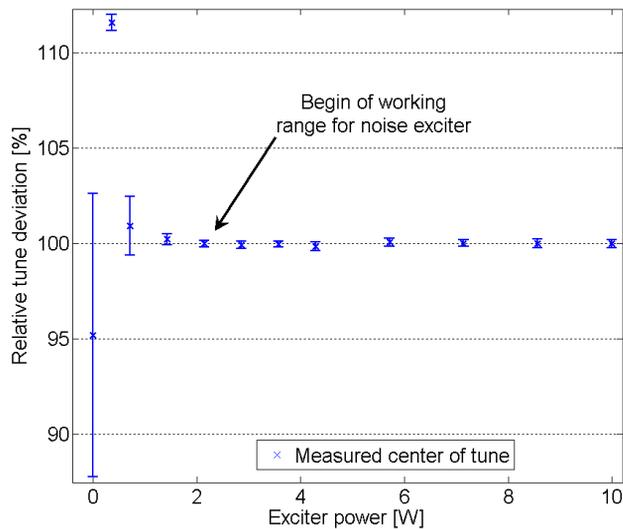
Figure 4: Points represent the mean value of 50 tune spectra with equal time offset to ramp start. Due to the fluctuations of obtained tune at low excitation the exciter power needed for the working range can be defined.
