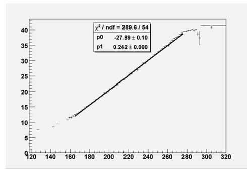
Figure 10: Muon range simulation in the EMR.  $\sum E$  vs Layer # is plotted. The horizontal axis is in MeV/c. Muons above  $\approx 270 \text{ MeV}/c$  will range through.
