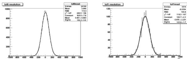
Figure 3: TOF0 detector's intrinsic timing.
