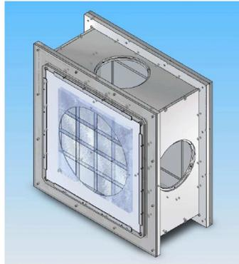
Figure 6: Model sketch of aerogel Cherenkov detector.
