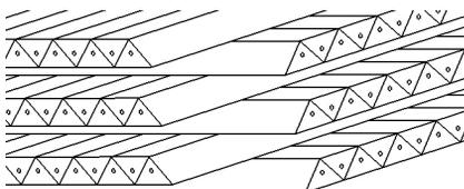
Figure 9: Sketch of MINERνA-like EMR calorimeter design to be used in MICE.
