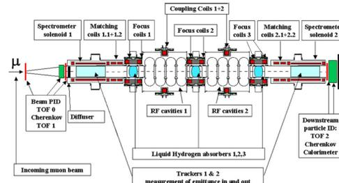
Figure 1: MICE Spectrometer Layout.
