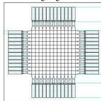
Figure 2: X/Y planes for TOF0 station. Each bar assembly is 4 cm wide.
