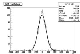
Figure 4: TOF1 detector's intrinsic timing.
