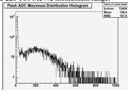
Figure 7: Typical light spectrum from single CKOV PMT, about 5-6 p.e. per channel  $\times 4$ .
