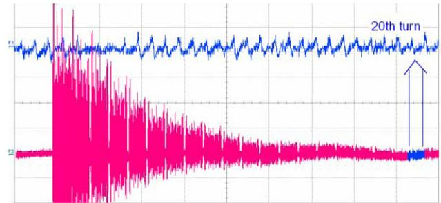
Figure 4: The stored beam signal from BPM in CSRm.
