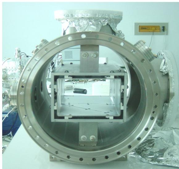
Figure2: The BPM structure of HIRFL-CSR.
