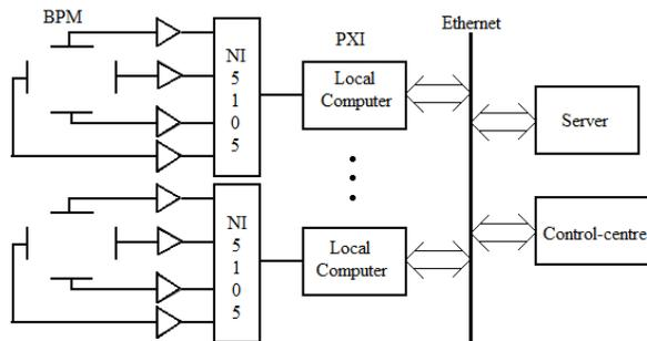
Figure 3: BPM processing system setup.
