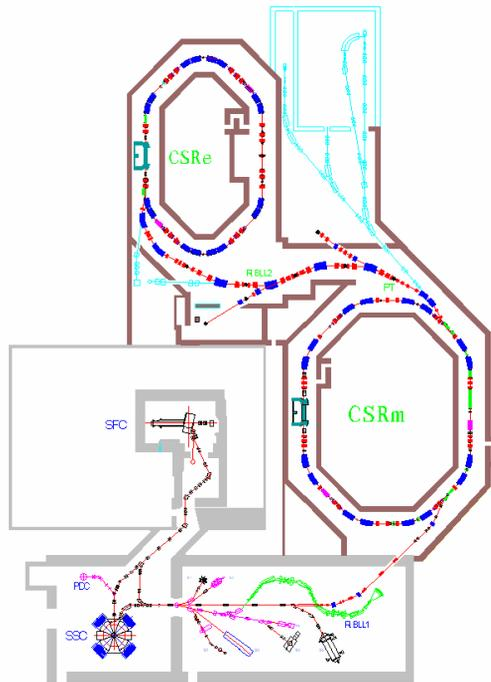
Figure 1: Overall layout of HIRFL-CSR.
