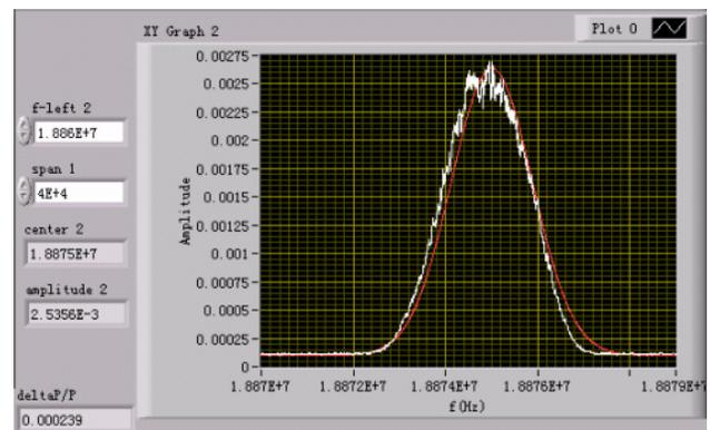
Figure 6: Momentum dispersion measurement in CSRc.
