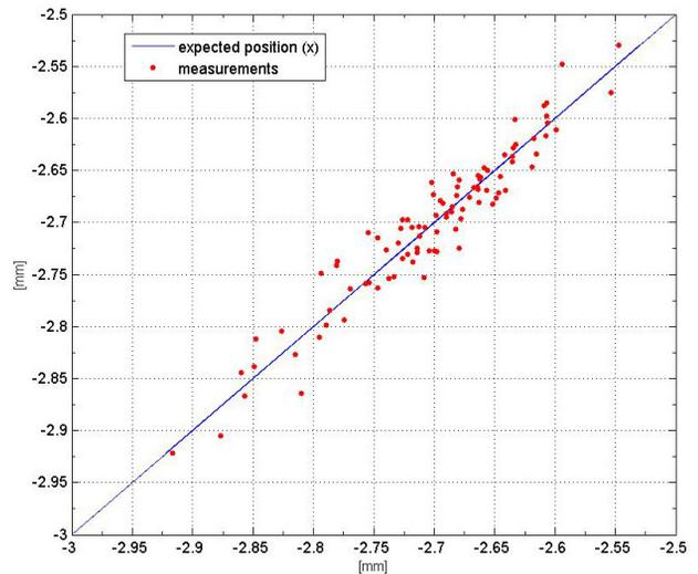
Figure 8: Expected horizontal position vs. measured position for the BPSTT03 BPM in the DAFNE transfer line.
