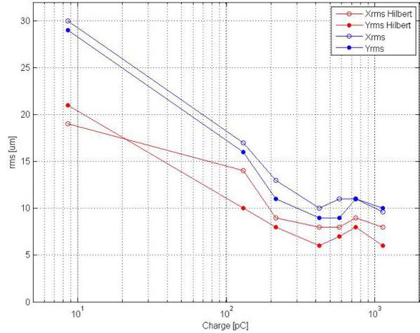
Figure 4: Measured resolution vs. bunch charge at Elettra.
