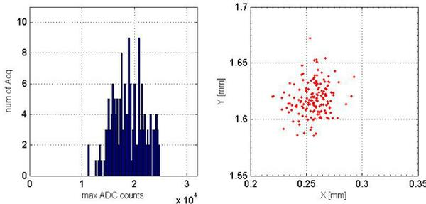
Figure 2: Histogram of maximum of ADC counts (left) and beam position (right) at a particular BPM at SPARC.
