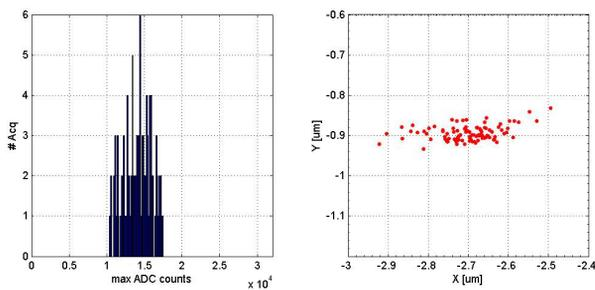
Figure 6: Histogram of maximum of ADC counts (left) and beam position (right) at a particular BPM in DAFNE.
