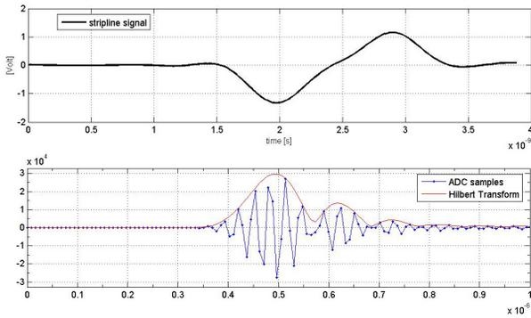
Figure 1: SPARC BPM signal (top) and Libera ADC sampled waveform (bottom), along with the computed Hilbert amplitude.
