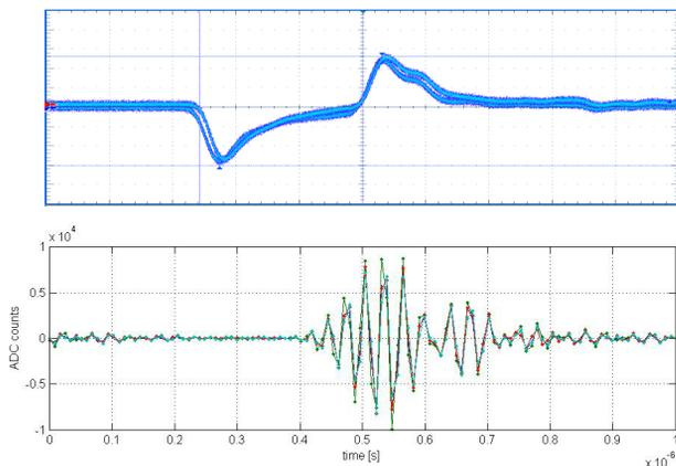
Figure 3: Stripline BPM signals at Elettra [400 mV/div vs 400 ps/div] (top) and Libera sampled data (bottom).
