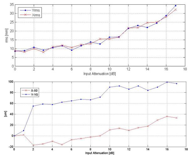
Figure 5: Position linearity (bottom) and resolution (top) vs. Libera input signal attenuation.
