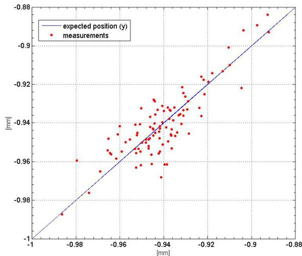
Figure 7: Expected vertical position vs. measured position for the BPSTT03 BPM in the DAFNE transfer line.
