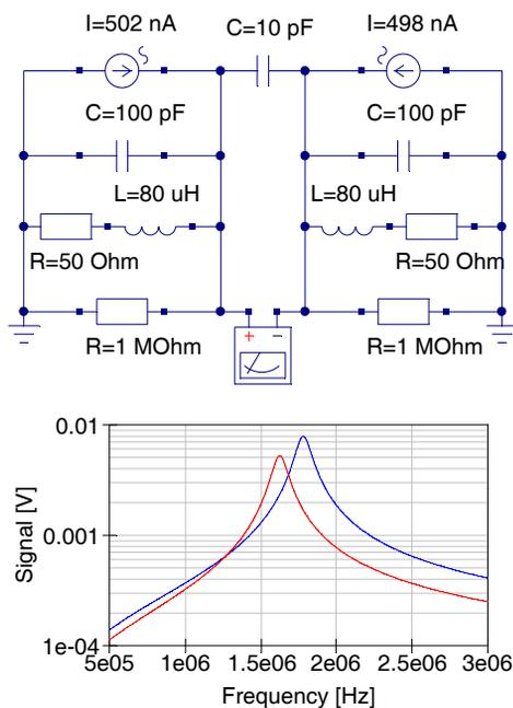
Figure 5: Equivalent circuit of two plates of the resonant capacitive PU and the resulting signal: peak voltage (blue curve) and differential voltage scaled by a factor of 100 for the picture clarity (red curve).
