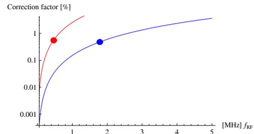
Figure 6: Correction factor calculated for 300 keV (blue) and 20 keV (red) bunches as a function of their repetition frequency (dots correspond to harmonic mode  $h = 10$ ).
