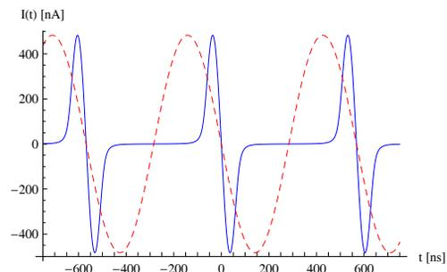
Figure 4: Image current flowing from the pick-up into an external circuit (blue curve) and a sine function with the same amplitude and repetition frequency (dashed red curve). The signal is generated on a PU plate of  $l = 100$  mm and  $r = 125$  mm by  $\cos^2$ -like bunches with  $\beta = 0.025$  and  $T = 150$  ns.
