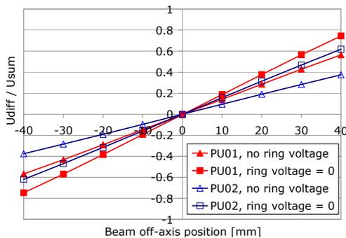
Figure 2: Response curves for two exemplary PU geometries with (squares) and without (triangles) ground voltage set to a guard ring introduced between PU plates.
