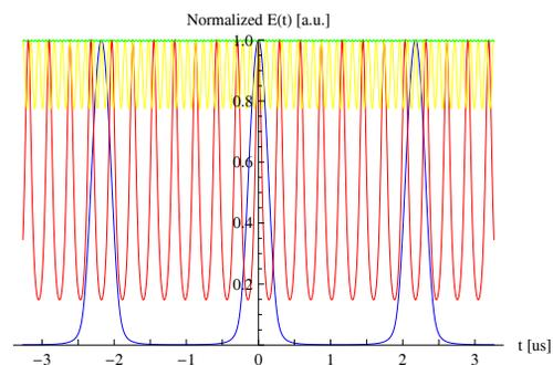
Figure 1: Normalized transverse electric field at a distance of 125 mm from the 20 keV  $\cos^2$ -like bunches formed with  $h = 10$  (460 kHz, blue curve), 75 (3.5 MHz, red curve), 200 (9.2 MHz, yellow curve), and 436 (20 MHz, green curve).
