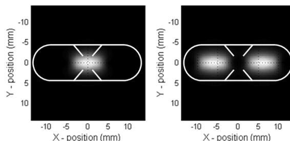
Figure 2: A standard four blade XBPM with the light from a normal ID (left) and light from two canted IDs (right). In this example the light from the two canted IDs has been normalised so they are of equal intensity.
