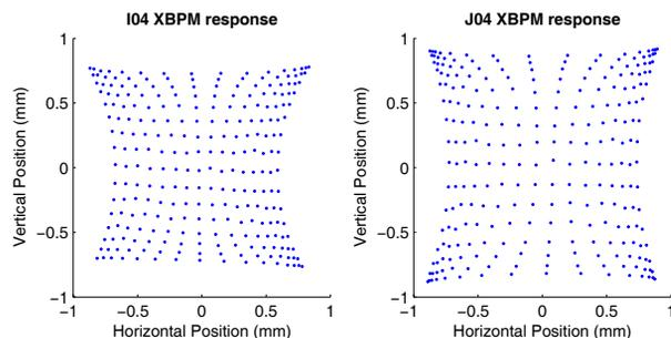
Figure 6: Response of the XBPM as the stepper motor position changes.
