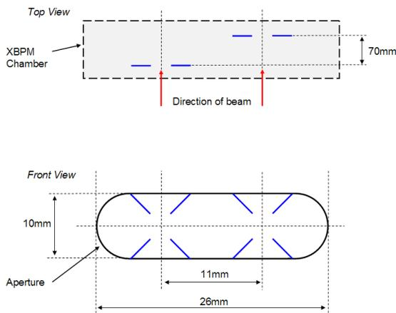
Figure 4: Dual beam XBPM schematic.
