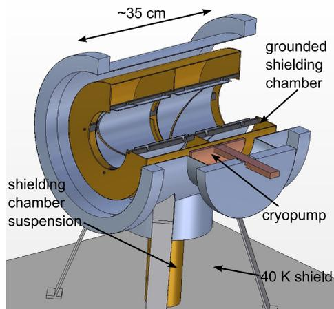
Figure 2: Preliminary mechanical design of the beam position monitor.
