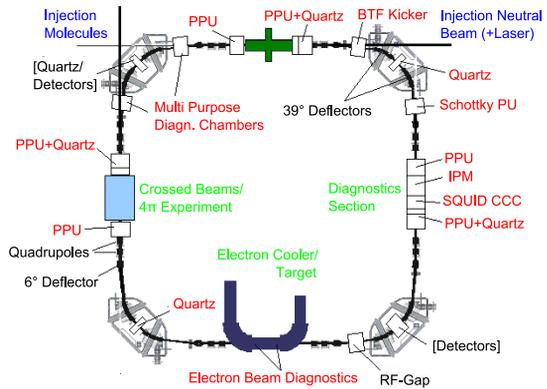
Figure 1: Overview over the CSR beam diagnostics system.
