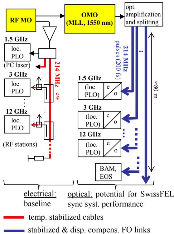
Figure 2: Simplified layout of electrical and optical reference distributions for the PSI 250 MeV Injector.
