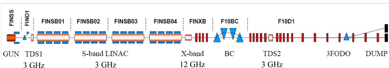
Figure 1: Simplified layout drawing of the PSI 250 MeV Injector [1].
