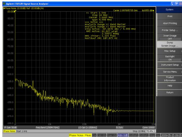
Figure 5: Measured phase noise of Onefive Origami 15 Soliton laser ( $\square f=1$  kHz..10 MHz,  $f_0=2.998$  GHz= $14^{\text{th}}$  harmonic of rep. rate 214.14 MHz): Setup (top), phase noise spectrum, timing jitter of 3.3 fs (bottom).
