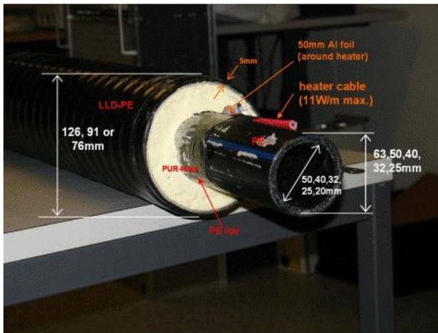
Figure 3: Temperature controlled cable pipe.
