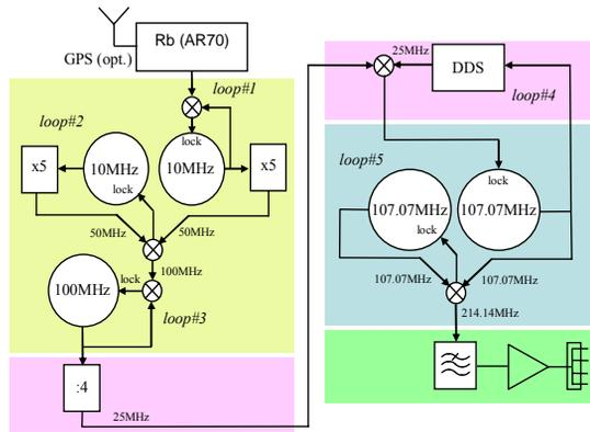
Figure 4: Block diagram of the RF master oscillator (214.14 MHz) [3].
