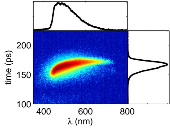
Figure 1: SC image presenting the pulse profile vs. wavelength. The chirp induced by the dispersion in the glass element traversed by the photon beam is clearly visible. The net result is a pulse broadening.
