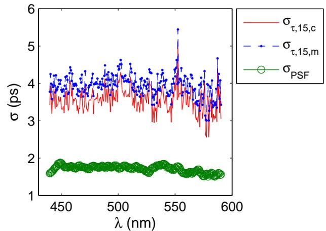
Figure 4: Pulse duration in the time-resolved spectrogram. The curves show measured and corrected r.m.s pulse width vs. wavelength. The relative spectrum intensity is shown in the inserted graph.
