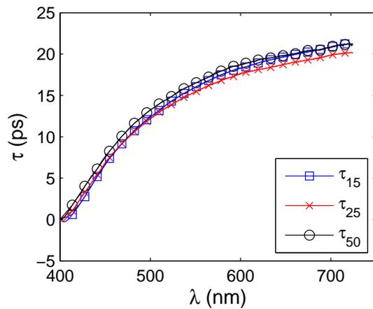
Figure 2: Centroid of the pulses vs. wavelength measured on Figure 1.  $\tau_{ii}$  indicates the sweep speed. Fit of the curves converges to the second order polynomial:  $y = -0.00026(\lambda - 400)^2 + 0.14(\lambda - 400) + 0.4$  ( $\lambda$  in nm and  $y$  in ps).
