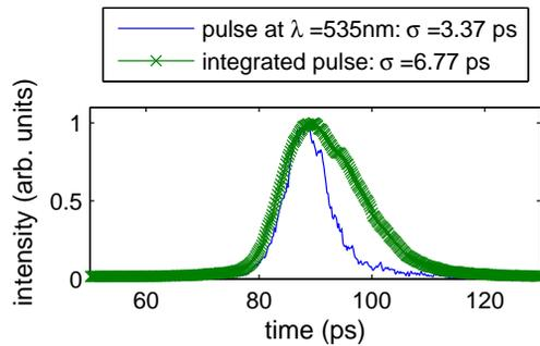
Figure 3: Pulse profile at 535nm compared to the integrated pulse over the spectrum.
