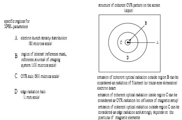
Figure 2: Scheme of the coherent OTR radiation pattern as observed in the object plane for the low electron beam energy case of 2 GeV.
