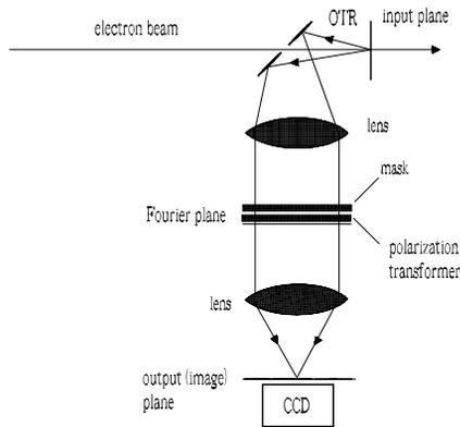
Figure 3: A practical arrangement of the coherent OTR image-processing system. (The hole in the OTR screen is for simplicity of drawing only. A tilted configuration should be used at these wavelengths instead.)
