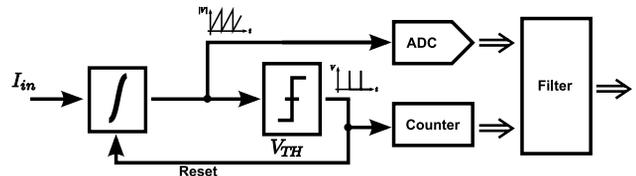
Figure 1: General scheme of a recycling integrator.
