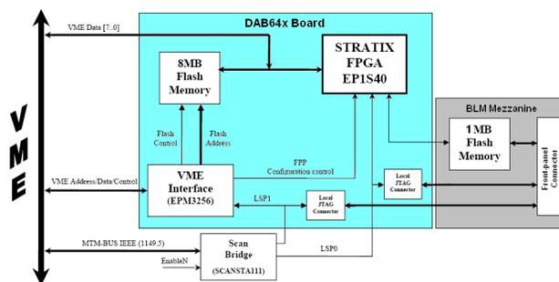
Figure 1: Block diagram of the FPGA firmware deployment and initialisation options.
