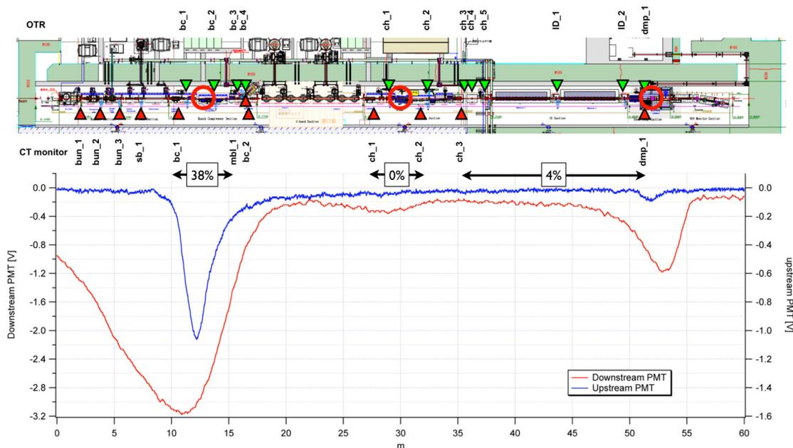
Figure 5: A typical beam loss measured on the SCSS prototype accelerator (single shot). Top: View of the SCSS accelerator with the location of the OTR and CT monitors (green and red triangles respectively). Bottom (b): The signals from the upstream and downstream PMTs. The percentages give the beam losses as measured by the CT monitors. The red circles indicate the position of the loss points.
