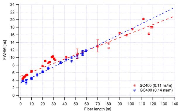
Figure 3: FWHM of the PMT signal as a function of the fiber length.
