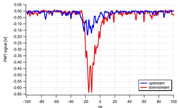
Figure 4: Beam loss signal (Fujikura SC400, single shot, 2.5 GS/s). The fiber is set so that the PMT is located 120 m upstream/downstream from the loss point.
