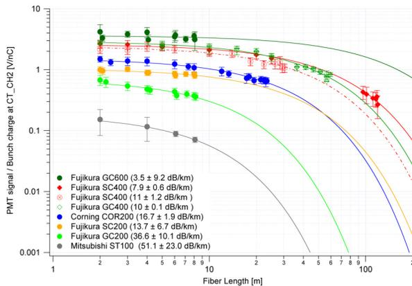
Figure 2: Signal from the PMT normalized by the average beam charge impacting the OTR screen as a function of the fiber length. The legend gives the values of the attenuation obtained from the fits.
