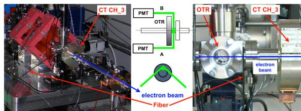
Figure 1: Experimental set-up used for the measurement of the attenuation of the beam loss monitor.
