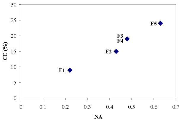
Figure 3: Collection efficiency of Cerenkov photons as a function of the Numerical Aperture (NA) of the optical fibres listed in Table 1. The collection efficiency is independent of the value of the fibre core diameter as it can be seen from the points F3 and F4.
