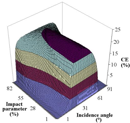
Figure 2: Collection efficiency of Cerenkov photons inside a pure silica optical fibre with NA=0.63.
