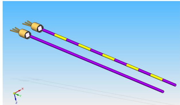
Figure 4: Sketch of the complete arrangement of the optical fibre sensor.
