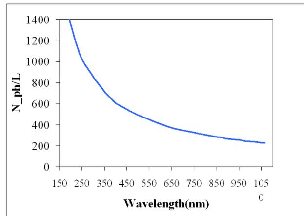
Figure 1: Number of photons produced per incident electron and per unit length  $L$  between 193 – 1064 nm.
