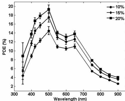
Figure 6: Photon detection efficiency of a SiPM as a function of wavelength (courtesy of ST-Microelectronics, Catania).
