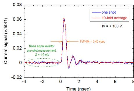
Figure 5: Pulse shape of the beam halo monitor (blue line: 10-fold average, red line: one shot measurement).
