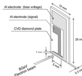
Figure 1: Structure of the diamond detector.
