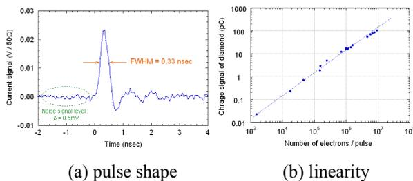
Figure 2: Measured data of the diamond detector.
