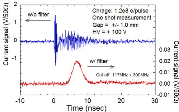
Figure 6: Effect of induction current and the suppression (upper: without LPFs, lower: with LPFs).
